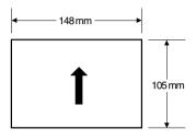
The figure below shows how much of a A4-, LTR-, or LGL-size document the machine scans when faxing or scanning.
